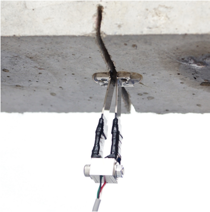
CMOD test, detail of clip gauge transducer (82-P0331/E)
