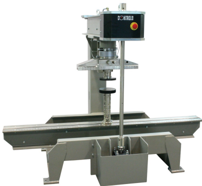
300kN UNIFLEX frame (50-C1601/FR) fitted with accessory for compression tests (50-C1601/4 and 50-C1601/KIT)
